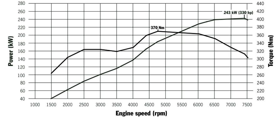
possible to achieve a power-to-weight ratio of less than 4 kg/hp. The light-alloy 3.4-litre horizontally opposed cylinder engine produces 243 kW (330 hp) at 7,400 rpm. Maximum torque is 370 Nm at 4,750 rpm.
